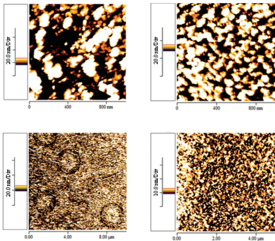
FIGURE 3. AFM morphology for ZnO-PANI/carbon black thin films with different weight ratio of ZnO (a) 0 wt%, (b) 4 wt%, (c) 6 wt% and (d) 8 wt%
