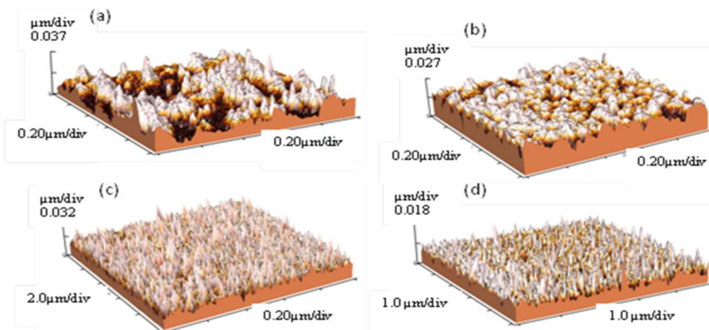
FIGURE 2. 3-D AFM image of ZnO-PANI/carbon black thin films with different weight ratio of ZnO (a) 0 wt%, (b) 4 wt%, (c) 6 wt% and (d) 8 wt%
