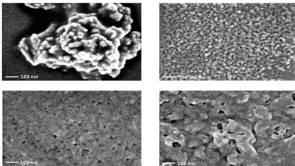
FIGURE 4. FE-SEM micrographs of ZnO-PANi/carbon black composite films for (a) 0 wt%, (b) 4 wt%, (c) 6 wt% and (d) 8 wt%
