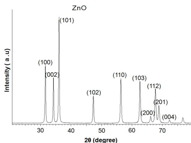
FIGURE 1. XRD result for ZnO powder
